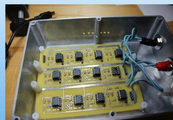
A PCB board was used to filter the Arduino's output in order to ensure the mirrors would not be damaged.
