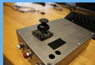
By changing the analog values (moving the joystick) it was possible to change the duty cycle of the pulse width which would effect the output voltage.
