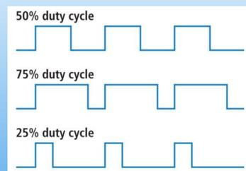
An Arduino is capable of outputting a pulse width modulation (PWM). The average value of the PWM is dependent on its duty cycle.
